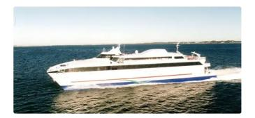
4 x MTU 16V 595 Diesels , 3,866 KW @1,770 rpm
